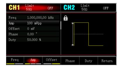
Press Freq key to set the frequency, use numerical keyboard to input 1 and then select the unit of parameter to kHz;
