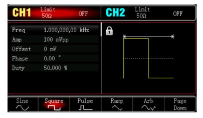
Press Amp soft key to set the amplitude, use numerical keyboard to input 1 and then select the unit of
